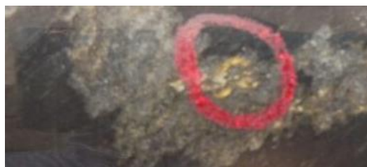
Figure 1: Visible gold (circled), several millimetres across, in a folded quartz vein in diamond drill core
